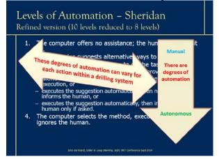
employed. These ranges will also transition from human control toward autonomous as automation is implemented. Understanding these stages provides a methodology to define the staircase toward autonomous operations and the role the human will play in various elements as the staircase progresses.
