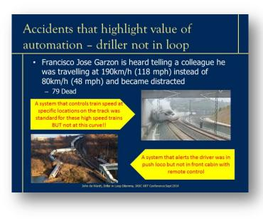
the tracks resulting in a major crash. The railroad system incorporated control systems that inhibited the high speed train from exceeding speed limits in critical sections of the track – except this one corner. If the system had been installed here, the train would have automatically slowed to the correct speed in spite of any distractions of the human operator.
